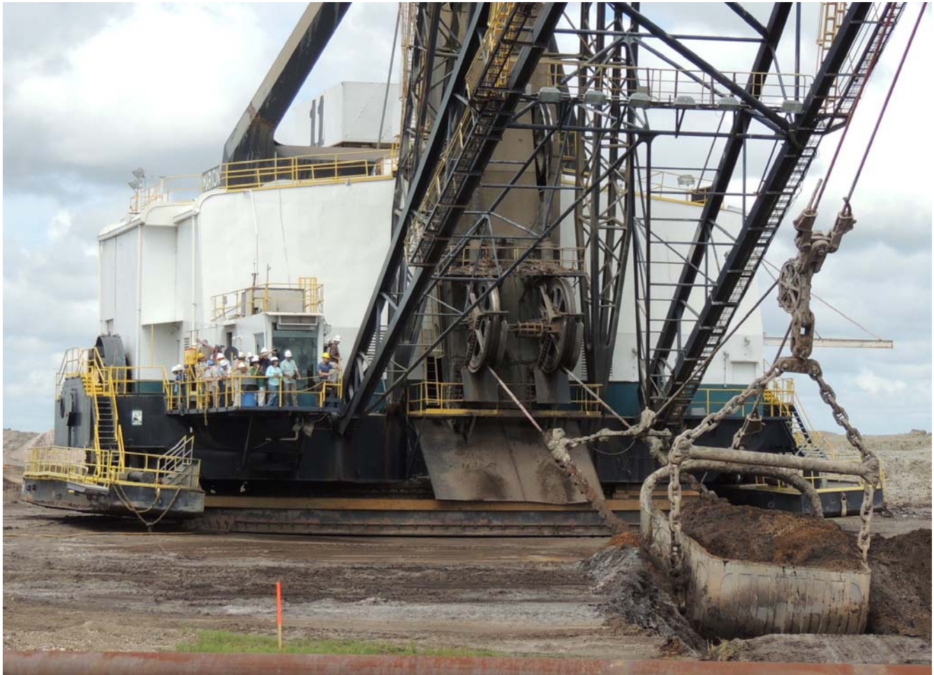
This is a Marion dragline with a 55 cubic yard bucket. Note the massive turntable, and the feet on either side used to "walk" the machine.
